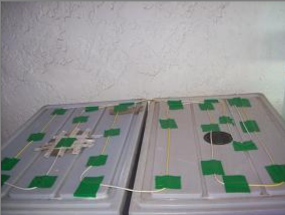
Picture of heating cable which heats each layer of drawers
